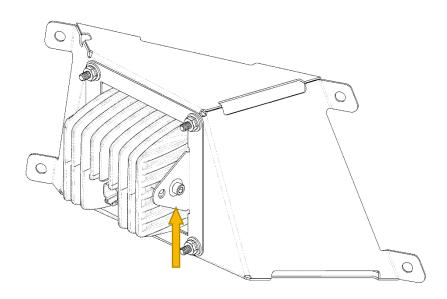
Light may be installed in either mounting hole depending on clearance behind bumper.
