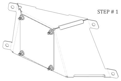
Remove blank plate with 5/32" hex driver and 7/16" drive socket.
